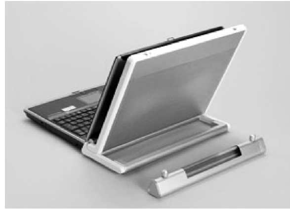
Fig. 4. Panasonic laptop with a DMFC powered by a methanol cartridge capable of a 20-h operation [29].
